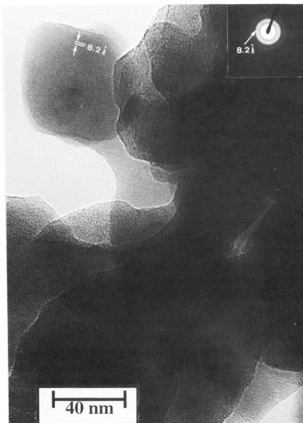
Figure 3. TEM bright field micrograph of pure fullerene powder.
